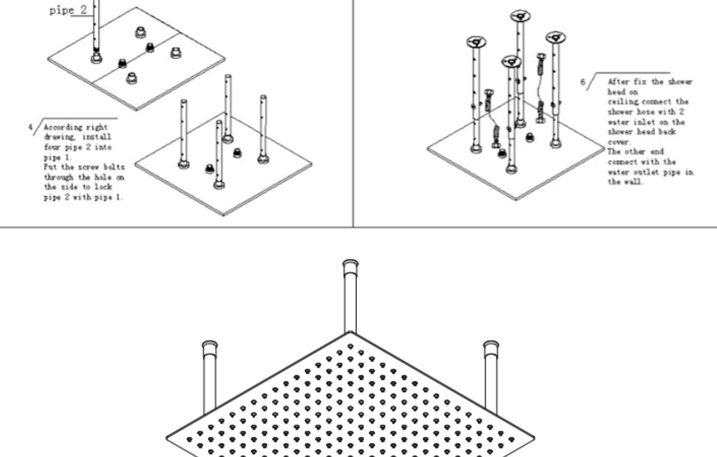
2, install fixing bar on ceiling
