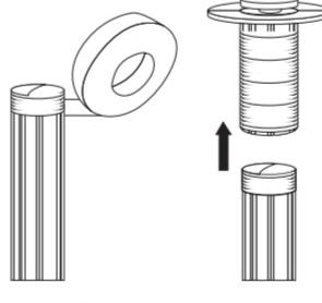
3. Slide the flat rubber gasket up the tailpiece until it meets the lip of the pop-up drain flange.
