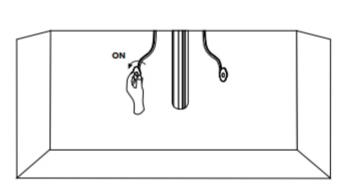
8. Proceed to sink drain installation. Once complete, turn the faucet on and check for leaks. Check to ensure that both hot and cold water are running properly. Allow the water to flow for approximately 60 seconds to remove any dust or sediment within the water lines.
