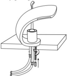
6. Apply plumber's tape or thread sealant to the threading on each braided water line. Attach the water lines to your main water supply. Ensure that you are connecting the hot and cold lines accordingly.
