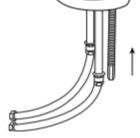
5. Secure the faucet by reattaching the brass lock nut that was removed in step 3. Hand tighten and adjust the faucet until it is properly aligned. Once aligned, finish firmly tightening the lock nut.
