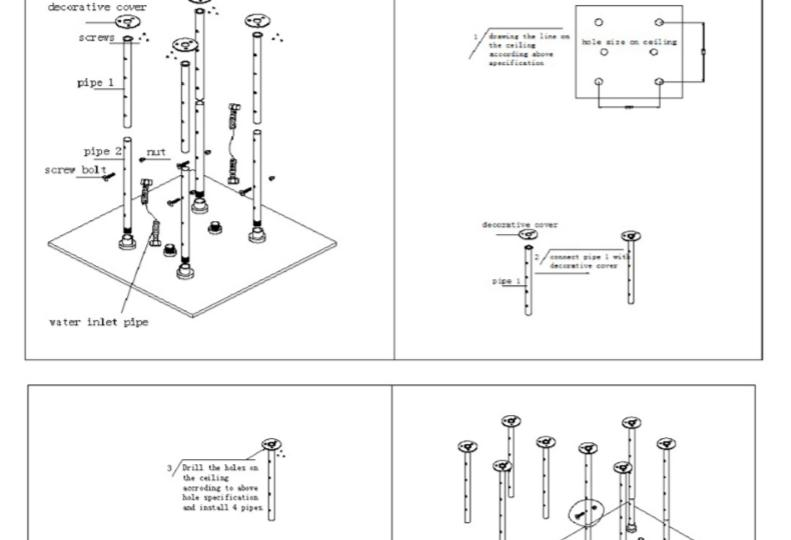
s right drawing shown, install four pipe 2 on the head
