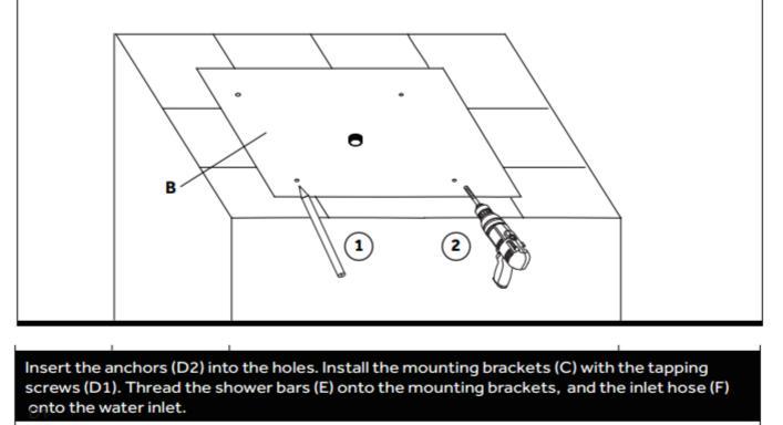
According to the template (B) mark the location of the mounting holes ①. Use a drill with a
