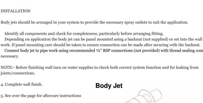
Installing the rough-in for the components. Decide how you want the functions to operate. I will describe this in more detail below. This is my recommendation.
