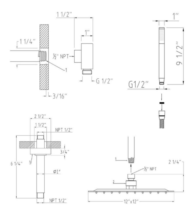
This general Diagram and installation are not intended for any specific model, but is presented as a general guide-line for installations!.
