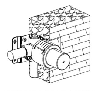
Put the protective cover on the valve body and finish the shower wall.
