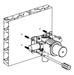
Install the valve body. Wrap the threaded portion of the joints in Teflon tape and connect the water inlet and outlet.
