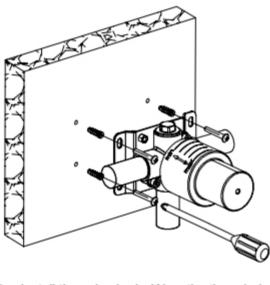
Install the valve body. Wrap the threaded portion of the joints in Teflon tape and connect the water inlet and outlet.
