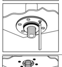
Mark the positions of four screw holes.
