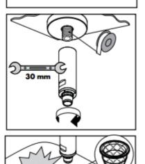
Wrap the threads on the nipple using Teflon tape.
