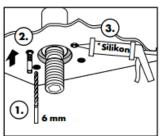
Drill the screw holes using a 6 mm bit (1).
