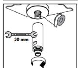
Wrap the threads on the nipple using Teflon tape. Install the extension pipe.
