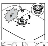
Make sure that the filter is installed in the showerhead. Push the showerhead against the extension pipe until it clicks.
