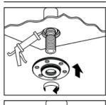
Seal the ceiling around the nipple using waterproof sealant.
