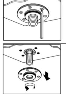
Drill the screw holes using a 6 mm bit (1).
